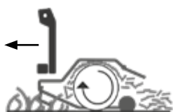
Open rear hood: mulching grass with low power consumption
